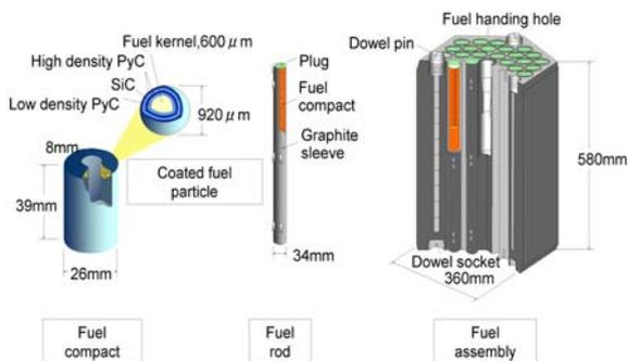
Fig. 4 Details of fuel structure of HTRR (by JAERI).
