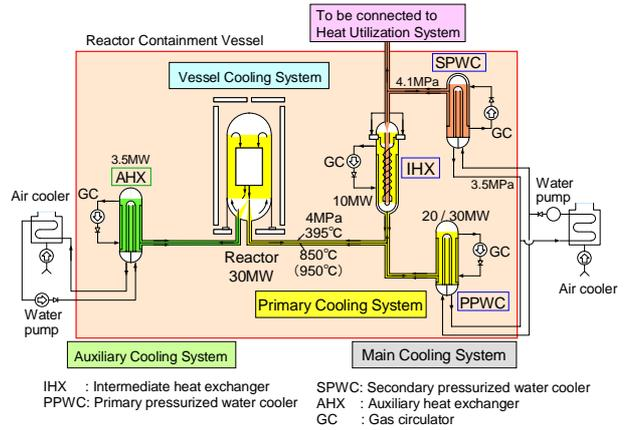
Fig. 5 Cooling system of HTRR of JAERI.
