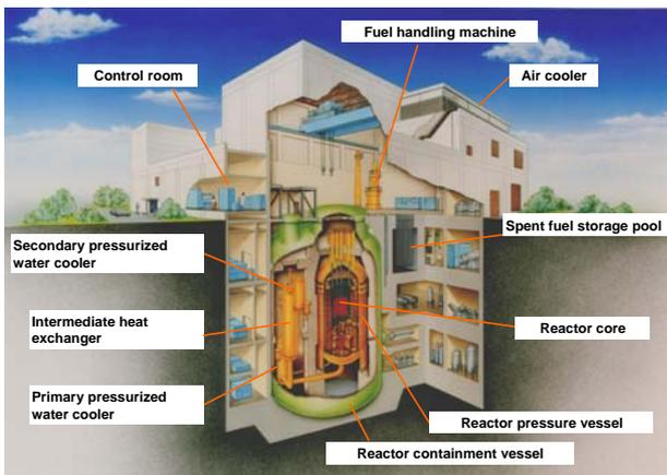
Fig. 3 Bird's-eye view of HTRR reactor building (by JAERI).
