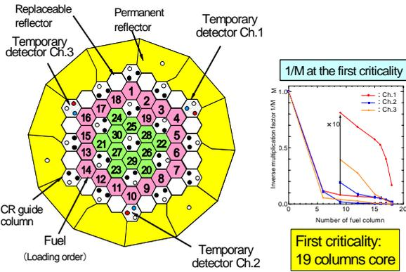
Fig. 8 First criticality at annular form of fuel loading in HTTR (horizontal cross section of core & fuel loading order).
