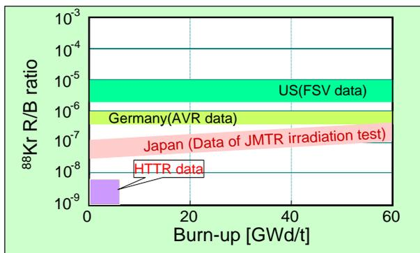
Fig. 10 Performance of coated particle fuel (by JAERI)
