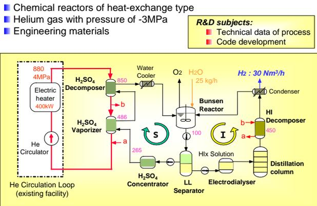
Fig. 20 IS process pilot test in JAERI.
