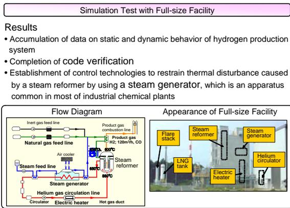
Fig. 21 System integration tests with steam reforming in JAERI.
