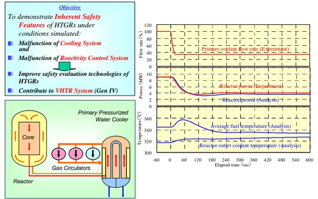
Fig. 11 Safety demonstration test using HTTR (Coolant flow reduction test).
