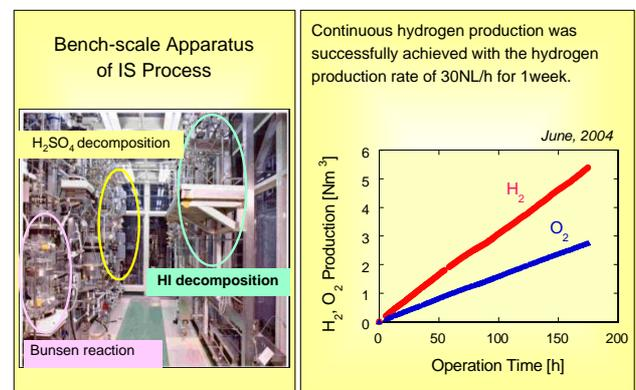
Fig. 19 Bench-scaled test result of IS process in JAERI.
