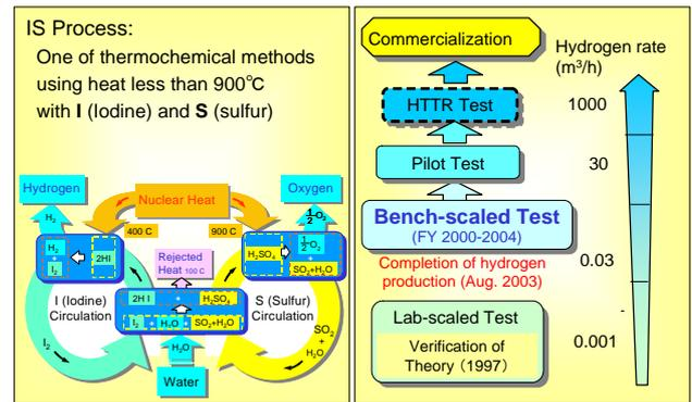
Fig. 18 Thermochemical hydrogen production process: IS process (JAERI).
