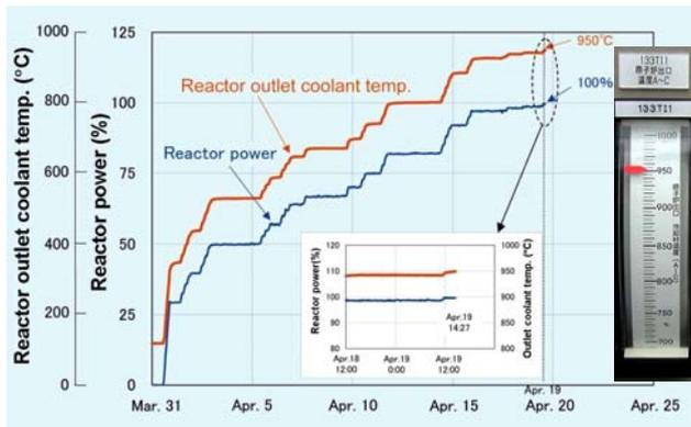
Fig. 9 Achievement of 950°C at reactor outlet of HTTR JAERI.
