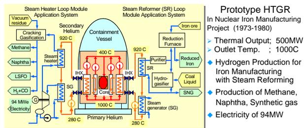
Fig. 1 Prototype reactor system of HTGR for multipurpose use designed in 1970s.
