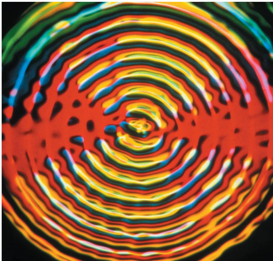
A Schlieren photograph — which shows density changes in fluids — of ripples in mercury.
